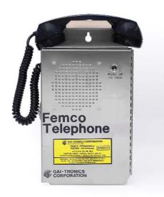
The LST operates from two 12 volt DC batteries which are placed in parallel during normal conversation to share on battery drain. Provisions on the LST unit keep the speakers quiet when receiving a normal audio signal or when paging. Input phone line DC polarity does not have to be observed since the unit design provides for polarity reversal.
